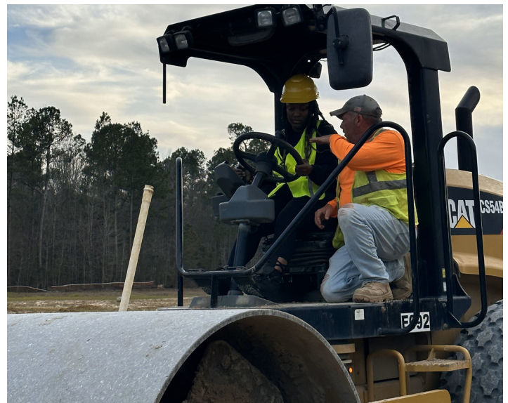
TCTP Charleston Instructor Jeff Luchini (right) of SC Safety Compliance explains the mechanics of the drum roller to TCTP participant Ms. ShaPerria Heyward who was later able to compress freshly laid loose dirt into a firm compaction.
